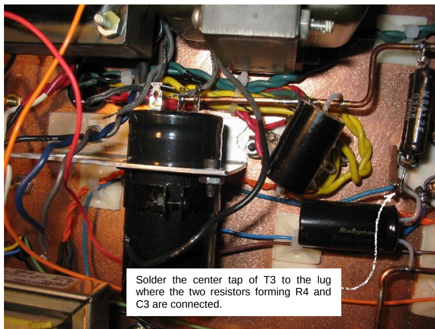
Figure 44. Connecting the center tap of T 3 to R 4 .
