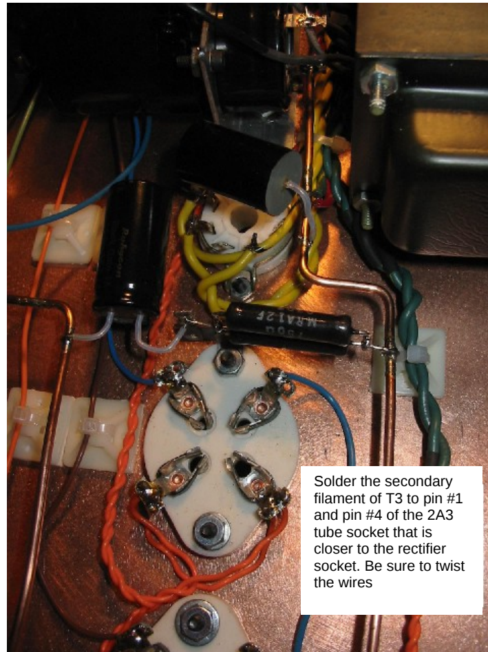
Figure 43. Soldering the secondary winding of T 3 to the rearmost 2A3 socket.
