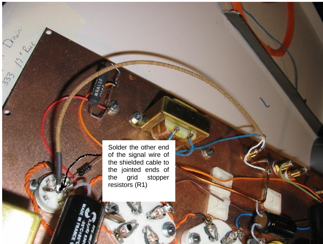
Figure 40. Soldering the input cable to the grid resistors ( R_1 )
