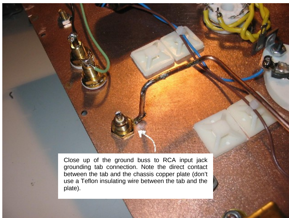
Figure 20. Detail of the ground buss connection to the RCA input jack.
