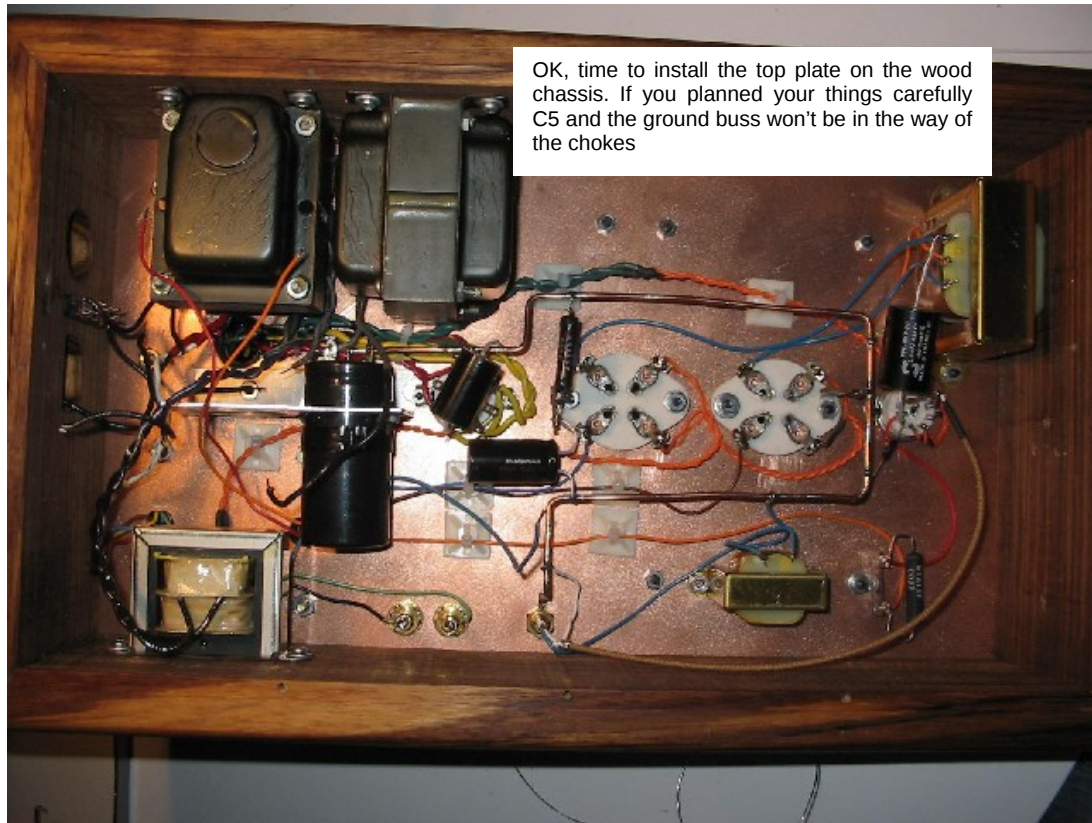
Figure 42. Installing the top plate on the chassis.
