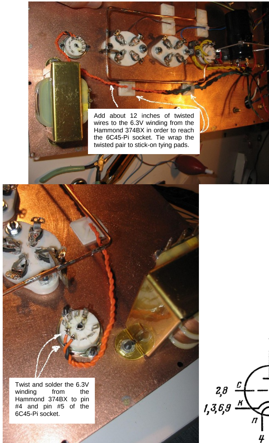
Figure 23. Wiring the 6.3V winding to the 6C45-Pi socket.
