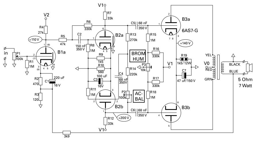
All resistors are 1 Watt Beyschlag resistors, unless otherwise noted VDV-6AS7: De Maurits; Copyright 1998 Menno van der Veen
