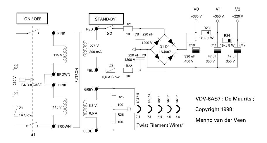
All resistors are 1 Watt Beyschlag resistors, unless noted otherwise
